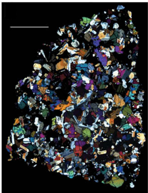
FIGURE 4.3 Photomicrograph of the EET 90020 basaltic eucrite, a differentiated meteorite thought to be derived from asteroid 4 Vesta. The scale bar is 2.5 mm. SOURCE: With kind permission from Springer Science+Business Media: H.Y. McSween, D.W. Mittlefehldt, A.W. Beck, R.G. Mayne, and T.J. McCoy, HED meteorites and their relationship to the geology of Vesta and the Dawn mission, Space Science Reviews , Online First, doi10.1007/s11214-010-9637-z, Copyright Springer Science+Business Media B.V. 2010.
