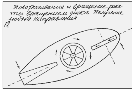
Fig. 8. Use of massive flywheels (gyroscopes) for rocket flight control.
