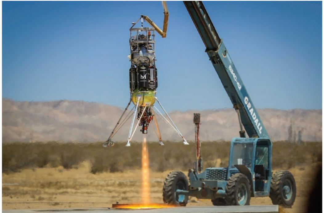
new planetary surface sampling technique, was successfully tested on a Xodiac rocket. This was a major step in moving a Planetary Society-supported project one step closer to flying in space someday. The Xodiac rocket lifted off, hovered and moved a short distance, and then landed PlanetVac in a bed of Mars
