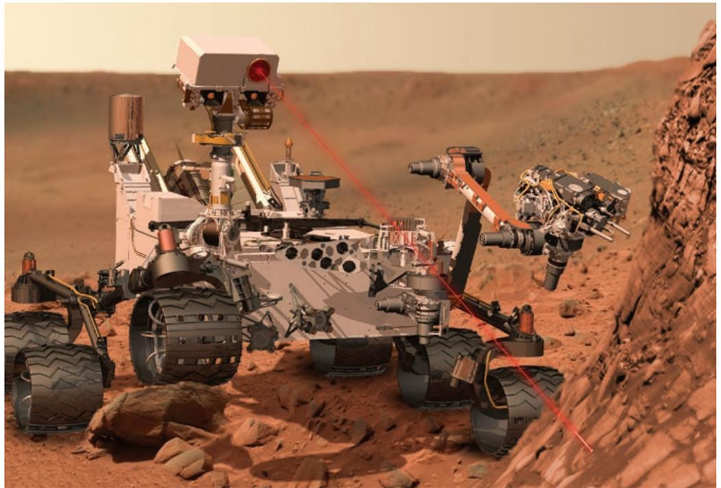
Exploration for Gathering Increased Science). The AEGIS software can analyze images from onboard cameras, identify geological features of interest, prioritize and select among them, and then point the rover's ChemCam instrument at selected targets to make scientific measurements.
