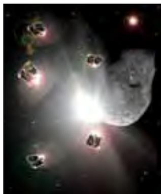
**CENTER** A very porous rock (top) and a less porous sandstone rock during laser ablation in the lab. Notice the conical plumes of material being ejected.
