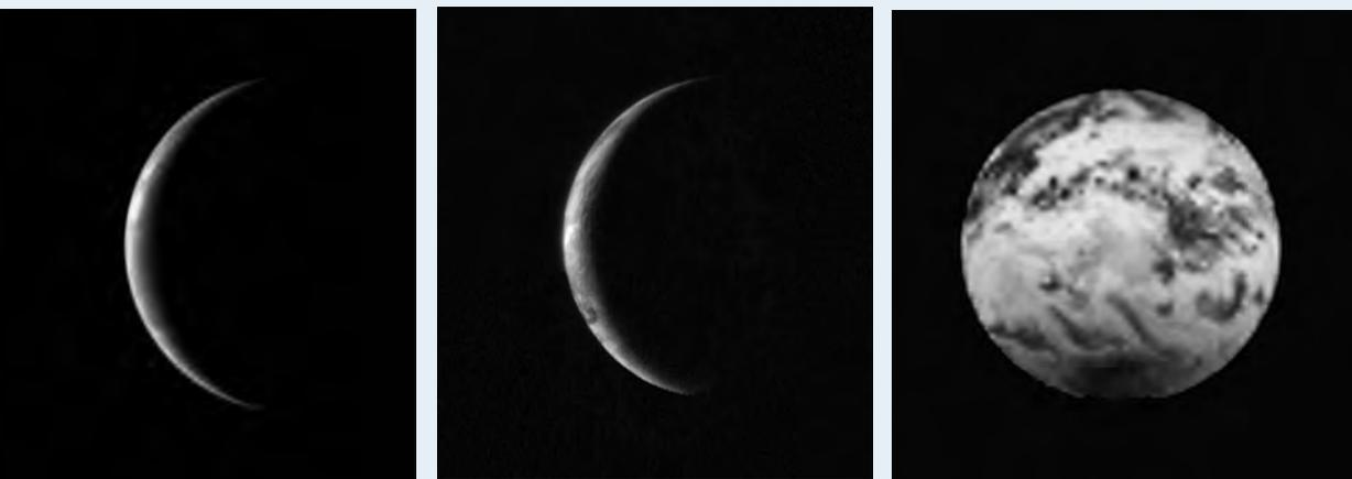
*Half a day after launch, Akatsuki team members tested the spacecraft's cameras on Earth. Taken at a distance of 250,000 kilometers (150,000 miles), the image at left shows how some solar radiation is reflected by clouds, while some is absorbed by the surface (center) and, finally, radiated back to space at infrared wavelengths. Thermal emissions from our planet's clouds and surface are evident in the image at right. Images: JAXA*
