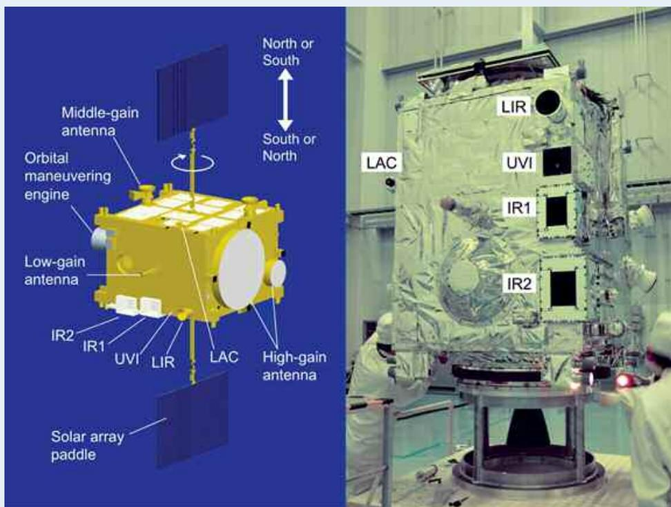
**Akatsuki’s cameras—specially designed for meteorological observations—will face Venus most of the time, while its solar array paddles are flexible about their north-south axis so that they can face the Sun no matter how the main spacecraft body is oriented. At right, engineers prepare to carry the spacecraft to the launch site. Graphic and photo: JAXA**
