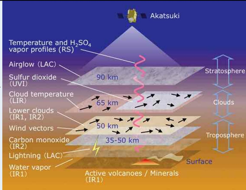
Data from Akatsuki's five cameras—which will include infrared imagery—along with radio occultation measurements will reveal the three-dimensional structure and dynamics of Venus' atmosphere. Graphic: JAXA
