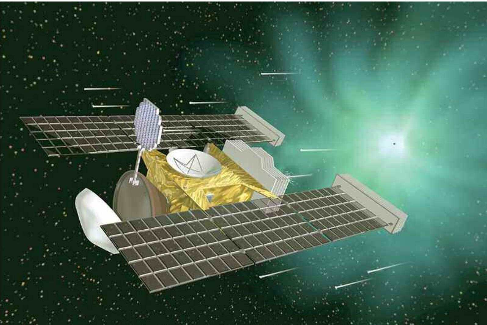
This artist's rendition of the Stardust spacecraft approaching comet Wild 2 shows the spacecraft in the process of collecting particles from the comet's coma by extending its paddle-shaped particle collector composed of ultralight aerogel. Using the reverse side of the collector throughout the spacecraft's 195-day journey to Wild 2, Stardust attempted to capture rare particles of interstellar dust. Orion may be prove to be such a particle. Image: NASA/JPL
