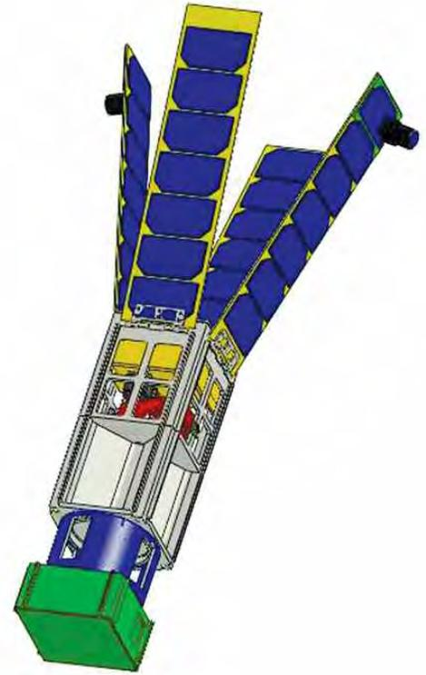
*The basic frame of LightSail-1's spacecraft is shown here. The cameras are the small black units mounted on the solar panels. The topmost CubeSat unit is the spacecraft bus (electronics, batteries, and antennas), and the bottom two CubeSats will house the folded sails and booms. Illustration: Chris Biddy, Stellar Exploration*
