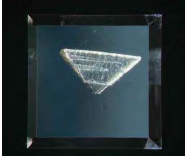
After a process of trial and error, the Stardust@Home team settled on this window as the optimal way to mount the pieces of the aerogel for study. In this configuration the "keystone" containing a candidate track is sandwiched between two silicon nitride windows, each only 70 nanometers in thickness.
