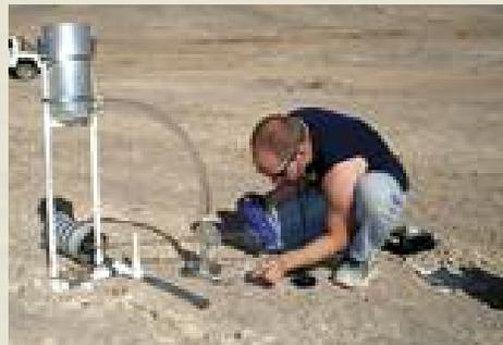
**THE PARAFFIN PLUG AROUND THE CONTACT HOSE MUST BE COMPLETE, OR AIR FROM THE RESERVOIR WILL ESCAPE IN UNKNOWN WAYS. WITH A COMPLETE CIRCULAR PLUG, THE FLOW OF GAS CAN BE MODELED AND THE SOIL'S PHYSICAL PROPERTIES CAN BE DETERMINED.**
