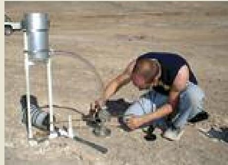
**TROY HUDSON POURS PARAFFIN AROUND THE CONTACT HOSE OF A SOIL PERMEAMETER. THE INSTRUMENT'S SILVER RESERVOIR AND "FLOAT" FORCE A STREAM OF AIR AT A CONSTANT PRESSURE INTO THE GROUND THROUGH A SURFACE PARAFFIN PLUG. THE RATE OF AIR FLOW INDICATES THE SOIL'S RESISTANCE TO FLUID MOVEMENT.**
