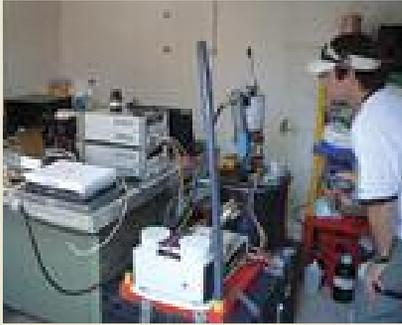
**IN THE MAKESHIFT LABORATORY, ANDREW AUBREY EXAMINES THE VORTEX COOLER ON THE SUBLIMATION OVEN, PART OF THE MARS ORGANIC DETECTOR, A HIGH-PRECISION SOIL ORGANIC EXTRACTION AND DETECTION SYSTEM. IT TOOK ABOUT 3 DAYS TO FULLY ASSEMBLE AND TEST THE INSTRUMENT.**
