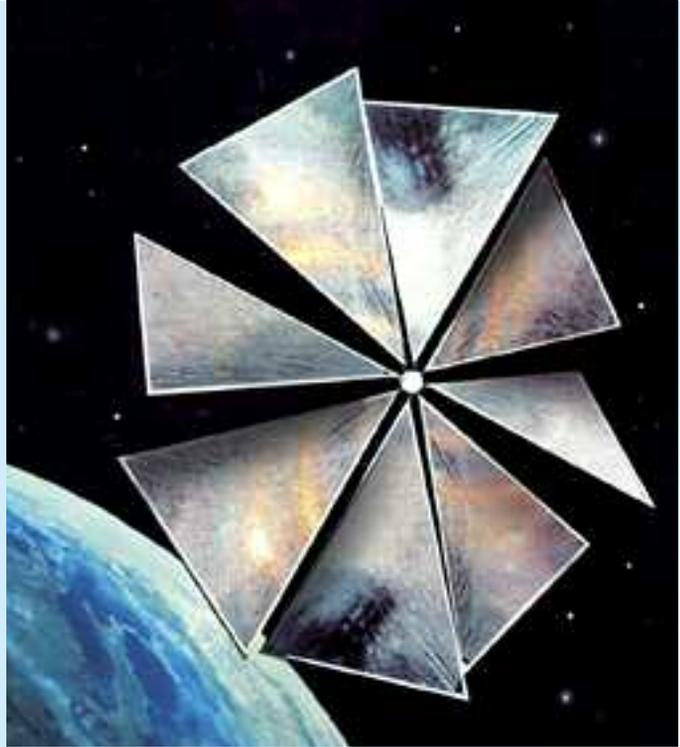
**Above:** In this illustration of *Cosmos 1* as it will appear in orbit around Earth, note the eight triangular blades, which can be rotated to face the Sun.
