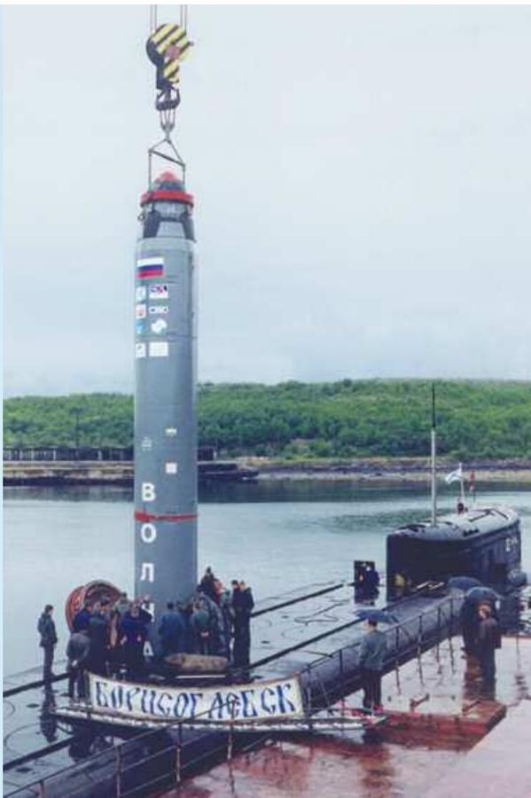
*The Volna rocket bearing the suborbital solar sail spacecraft was lowered into the submarine Borisoglebsk in July 2001. The suborbital flight was intended to test the deployment of the sails in a space environment. During the flight, a malfunction in the launch vehicle caused the spacecraft to remain attached to the last stage of the rocket, and the sails could not deploy. An identical Volna rocket will launch Cosmos 1 on its historic flight this winter. Photo: Makeev Rocket Design Bureau*
