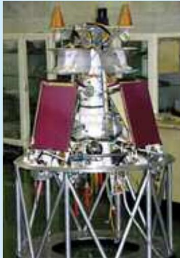
*This photo of the partially assembled Cosmos 1 spacecraft was taken in late October 2004 at NPO Lavochkin in Moscow. Note the folded solar panels (in red), which will be deployed in the first hour after the launch. In this view, the folded sails themselves have not yet been installed on the spacecraft. Photo: NPO Lavochkin*
