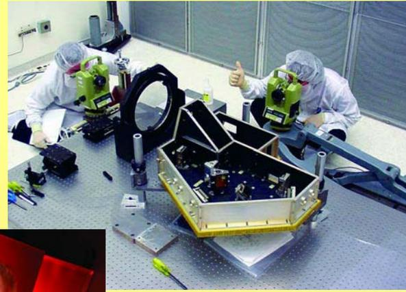
**Above:** Engineers align mirrors in the Spectral Imaging Module (SIM) of Deep Impact’s High Resolution Instrument. This instrument and the camera will watch the crater form and will measure spectral signatures of Tempel 1 before and after impact. These signatures will reveal the composition of the comet’s surface and interior.
