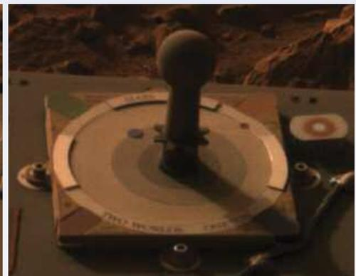
On September 25, 2004, the Mars Exploration Rover *Spirit* snapped its 50,000th image of Mars—then kept on snapping. The images above are of the Panoramic Camera's calibration target, also called the MarsDial. The 50,000th image (black and white) was taken as part of a sequence of images in a panoramic view of the Columbia Hills on *Spirit*'s 260th Martian day.
