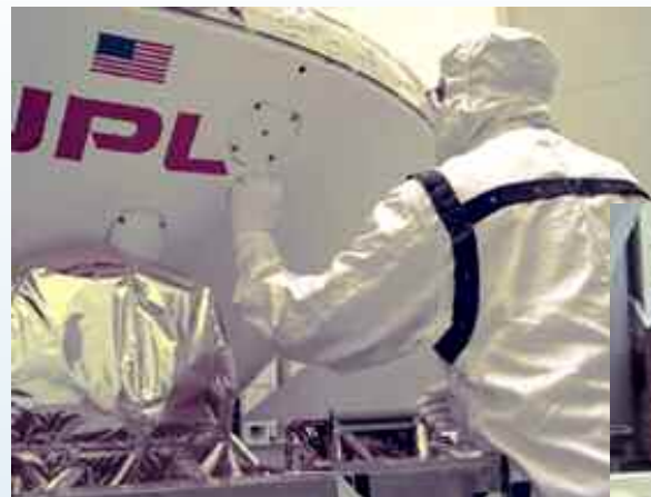
Before the Mars Exploration Rovers launched off the surface of the Blue Planet for their trip to the surface of the Red Planet, they had to be examined thoroughly to make sure they weren't carrying any unwanted microorganisms. Above: Larry Kirschner samples the outside of the backshell covering the encapsulated spacecraft; right: Bob Koukol and Lori Shiraishi perform microbiological sampling of the instruments and the Instrument Deployment Device.
