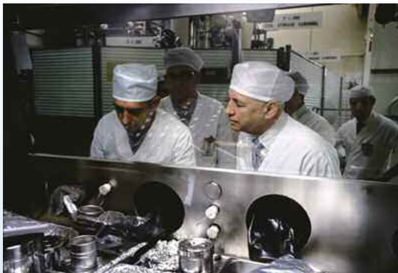
Rocks and "soil" returned from the lunar surface were treated with great care to ensure that they were not contaminated by Earthly organisms. These researchers, wearing germ-free clothing, are examining a sample from Apollo 17 that is inside a sterile isolation chamber. Photo: JSC/NASA
