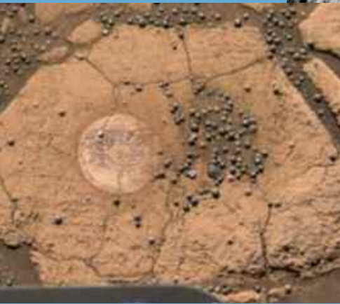
This true-color view shows the hematite concretions sitting on and around part of the outcrop in Eagle crater. The rover's rock abrasion tool (RAT) has left behind a shallow depression 5 centimeters (2 inches) across. Use of the RAT enables us to get below the weathering rind at the surface and place instruments on the underlying unaltered rock. Image: JPL/NASA
