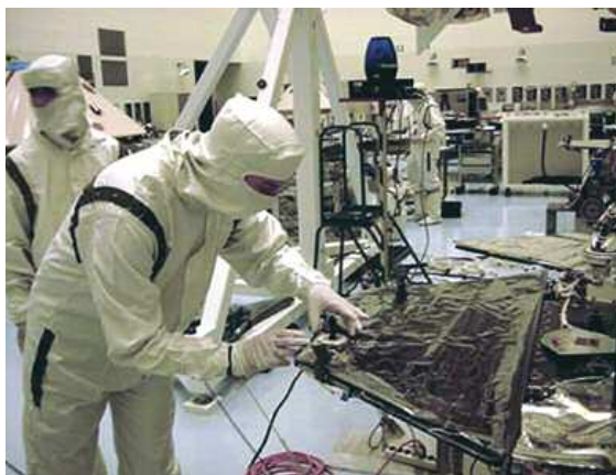
Jim Bell, one of the authors and Pancam Payload Element Lead, places the MarsDial on the rear solar panel deck of one of the Mars Exploration Rovers at the Kennedy Space Center. Photo: NASA/JPL/Cornell
