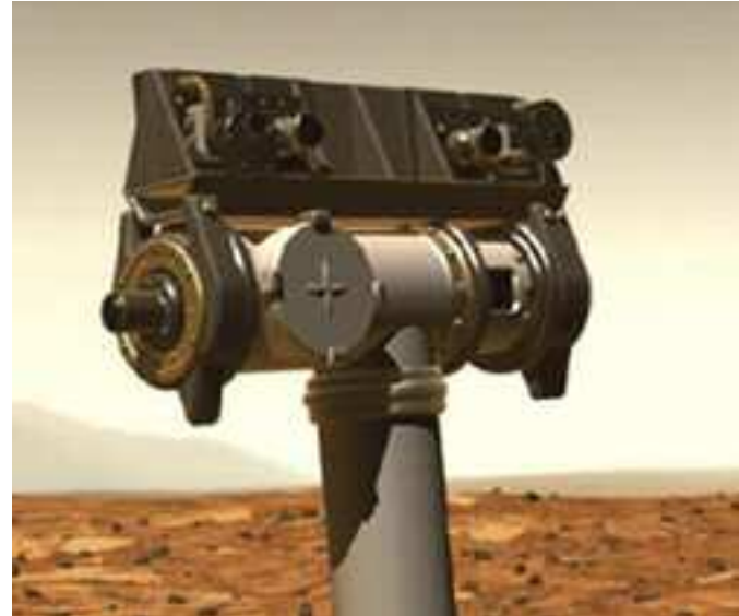
Above: Pancam has a camera bar that contains Pancam and Navcam (navigation camera) heads. Designed to "see" the way human eyes do, the cameras are mounted atop a mast about 1.5 meters above the surface, which allows Pancam a full 360 degree view. Additionally, each camera has the equivalent of 20/20 vision and a "visor" that changes the elevation of the camera so the rover can look up or down.
