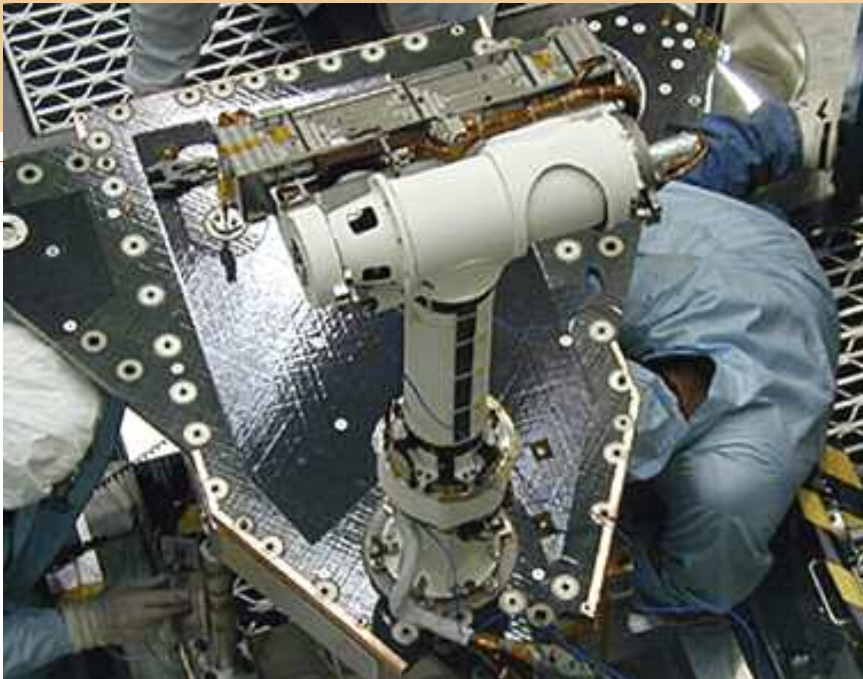
Above: This photo shows the Pancam's mast assembly with the camera bar in stowed position, ready for flight.
