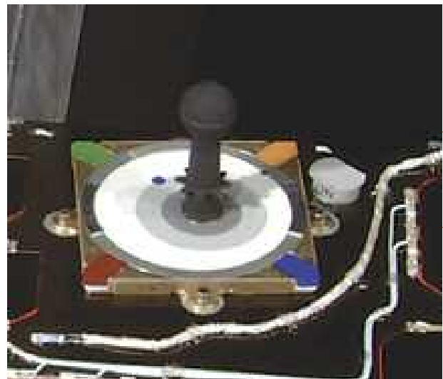
This color Pancam image of the MarsDial on the Opportunity rover during system thermal vacuum testing shows the size and orientation of the dial images expected to be returned from Mars. The multiple gnomon shadows are caused by multiple light sources in the vacuum chamber.
