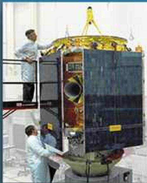
*Inset: Engineers prepare Near Earth Asteroid Rendezvous (NEAR) for loading onto a Delta 7925—the smallest rocket used to launch a planetary mission. In this photo the spacecraft's solar panels are folded down.*
