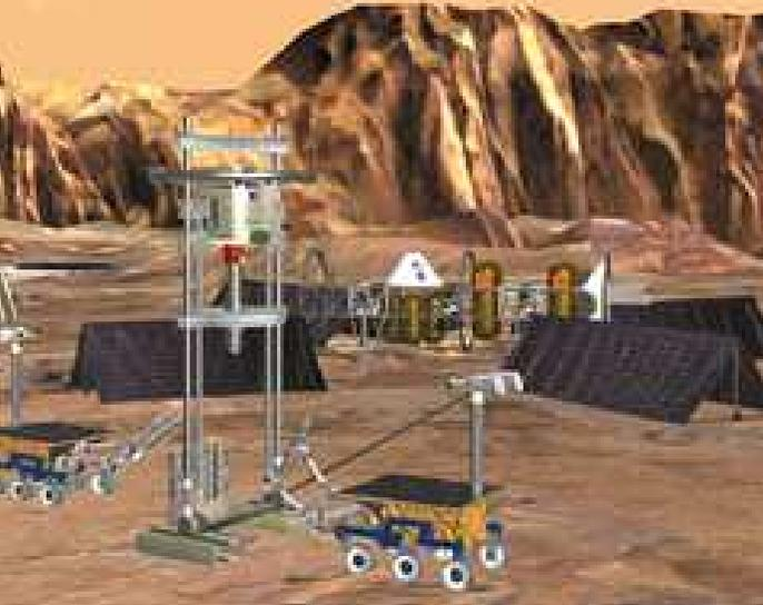
*The next logical step in Mars exploration is to establish a permanent presence on the planet. An early robotic outpost might look something like this: solar arrays surround a resource utilization system, while in the foreground two rovers assemble a drill. Illustration: JPL/NASA*
