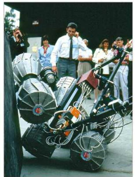
**Go figure!** The Mars Rover performed splendidly in all the tests we put it through. That is, until the day we trotted it out for NASA Administrator Daniel Goldin at the Jet Propulsion Laboratory. The rover's obstacle-avoidance computer program malfunctioned, and it contorted wildly trying to get past a barrier. That's Viktor Kerzhanovich wondering what went wrong. Photo: Charlene M. Anderson
