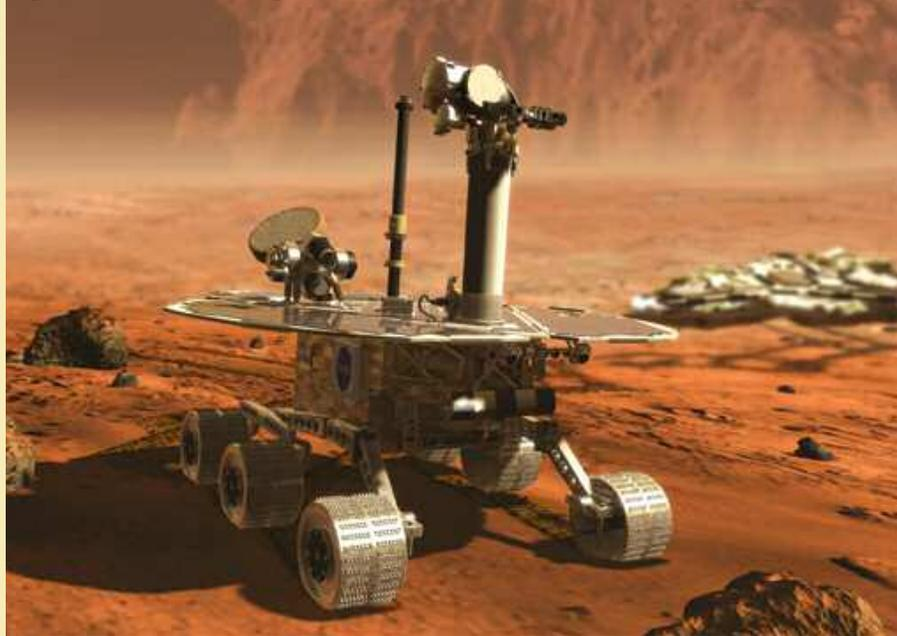
*Rovers are extremely efficient little explorers. This NASA illustration shows the Mars 2003 Rover as it sets off to roam the surface of the Red Planet. The spacecraft is scheduled to launch in June 2003 and will land on Mars in January 2004. Collapsed at right is the airbag shell that shielded the rover's landing. Illustration: JPL/NASA*
