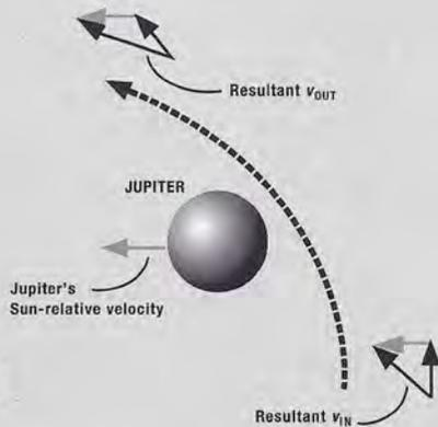
Figure 2. Jupiter is moving with respect to the Sun, and the spacecraft acquires some of Jupiter's velocity through mutual gravitational attraction. The result is that the magnitude of its outbound velocity,  $v_{OUT}$ , exceeds that of its inbound velocity,  $v_{IN}$ , relative to the Sun.
