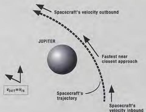
Figure 1. Relative to Jupiter, the spacecraft ends up with the same velocity,  $v$ , leaving as it had coming in, even though it accelerates during flyby.
