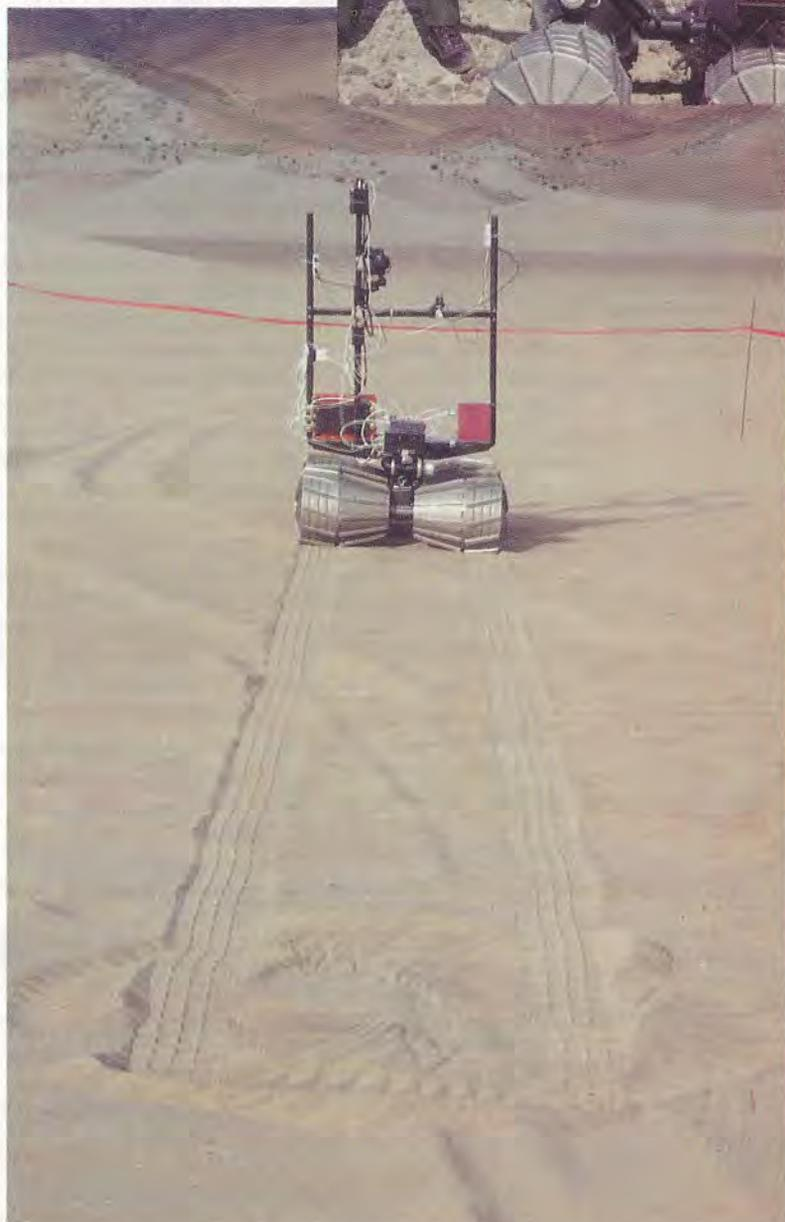
chassis of the Mars Rover on Kamchatka in 1991 was successfully carried out by our institute. And it was precisely the results of these and earlier tests that enabled us to prepare the Mars Rover for its successful operation in California.
