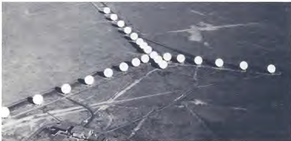
The Very Large Array in New Mexico (above) is a group of radio telescopes that can be used simultaneously to observe an astronomical object. By carefully combining the radiation collected by each individual dish, researchers can reconstruct an image as if the entire area enclosed by the array were a single, giant aperture. This technique has many advantages for detecting and characterizing extrasolar planets.
