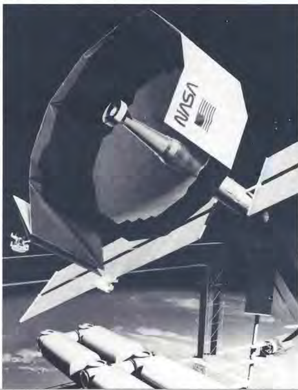
In this painting (right), NASA's Large Deployable Reflector, now being studied at the Jet Propulsion Laboratory, is constructed in Earth orbit. This type of telescope uses a segmented primary mirror to produce direct images of the source. This telescope is one possible approach to the problem of finding and studying extrasolar planets.
