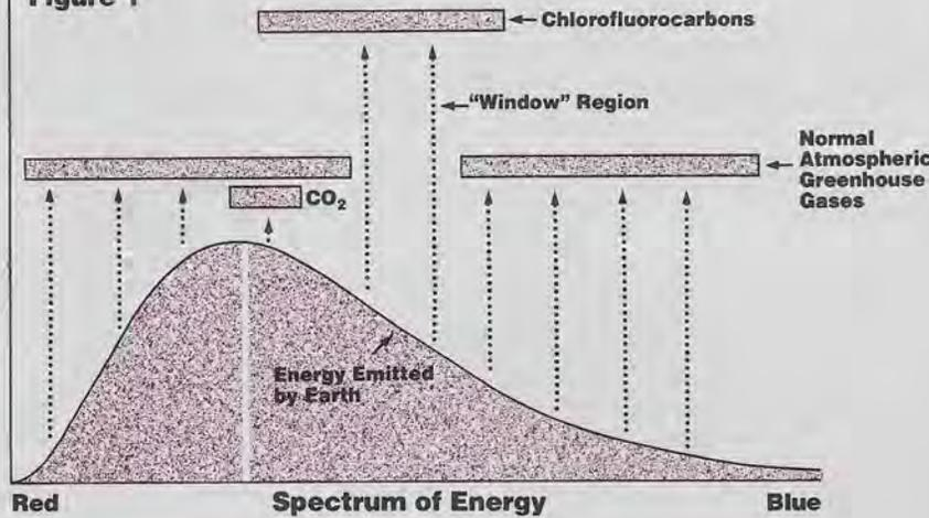
Greenhouse gases, such as water (H<sub>2</sub>O) and carbon dioxide (CO<sub>2</sub>) warmed the planets Venus and Earth and may someday help to warm Mars. This graph shows how the energy emitted by a planet can be trapped by the primary greenhouse gases. If future terraformers wanted to warm Mars "quickly," they might plug the spectral window where energy might escape by introducing chlorofluorocarbons into the martian atmosphere. Chart: S.A. Smith
