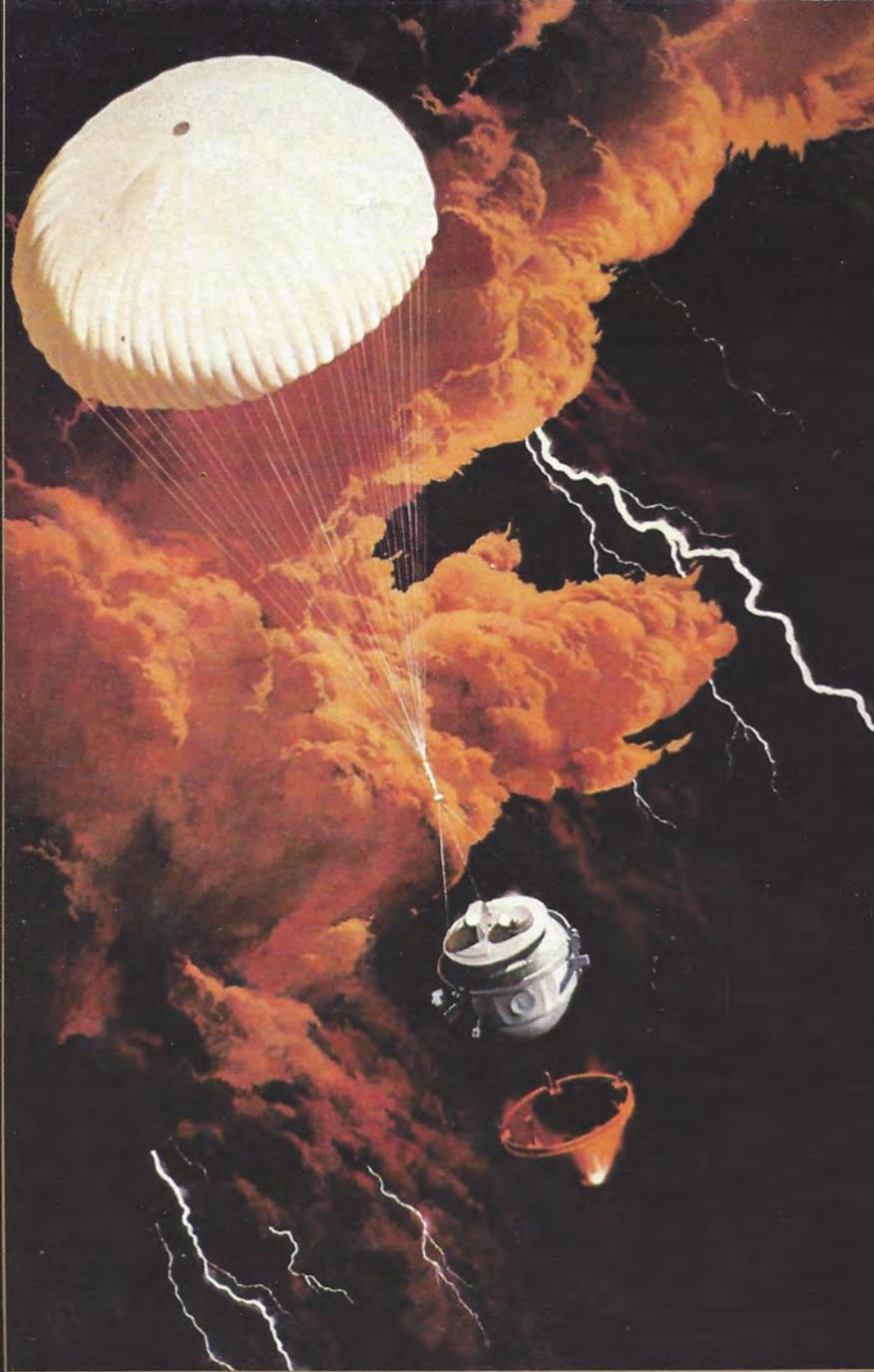
**GALILEO PROBE** — A parachute slows the Galileo probe as it enters the turbulent atmosphere of Jupiter. This probe is part of a two-pronged mission that will also send an orbiter to circulate among the jovian moons. Often postponed, the mission may now be launched in 1989 or the early 1990s.
