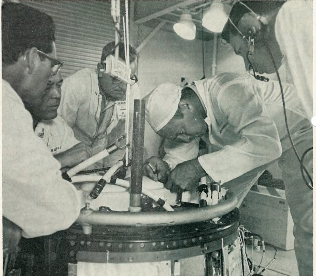
LIKE SKILLED surgeons, McDonnell technicians install test gear in the Gemini 6 nose tip for radar checks. The spacecraft went through weeks of pre-flight checkout at the Kennedy Space Center before being mated to its launch vehicle at Complex 19.
