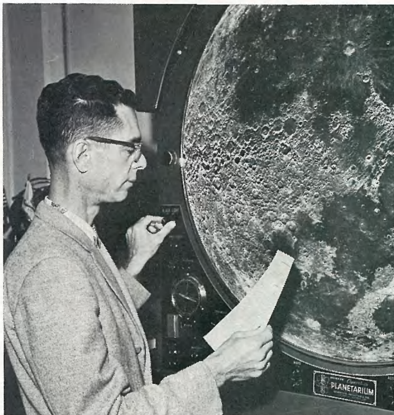
PLANETARY PLOTTER Lester Keene, LVOD Aerospace Technologist, checks chart with lunar landscape on this planetarium demonstration machine. Capable of demonstrating astronomical phenomena and planetary positions, past or present, the machine also shows planets and stars as points of light on its "wide screen" surface.
