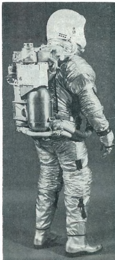
GEARED for a four-hour stroll on the lunar surface is this model, wearing a prototype of the space suit and life support pack being developed for the Apollo program by the Hamilton Standard division of United Aircraft. Rubber bellows at the joints of arms, legs and torso provide greatly increased mobility when the suit is pressurized.
