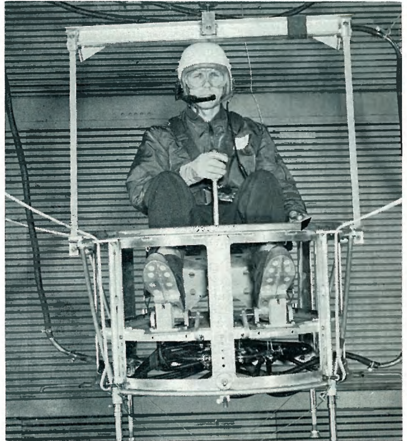
A TEST PILOT guides this weird-looking Lunar Research Vehicle toward a simulated moon landing. The "flying machine" is to be put through rigid tests at NASA's Langley Research Center.
