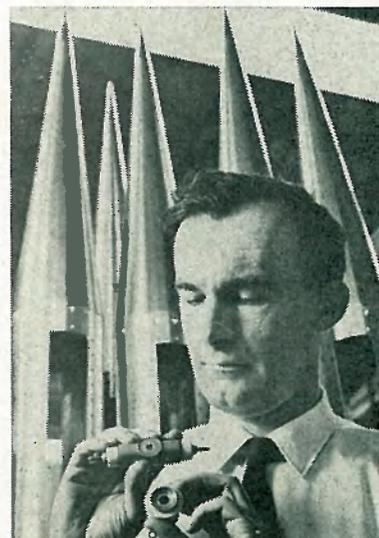
**DR. LESLIE SMITH** of the Geophysics Corp. of America holds solar radiation sensory instruments used on six Nike-Apache sounding rockets fired into the ionosphere from Ft. Churchill, Canada, during the solar eclipse.
