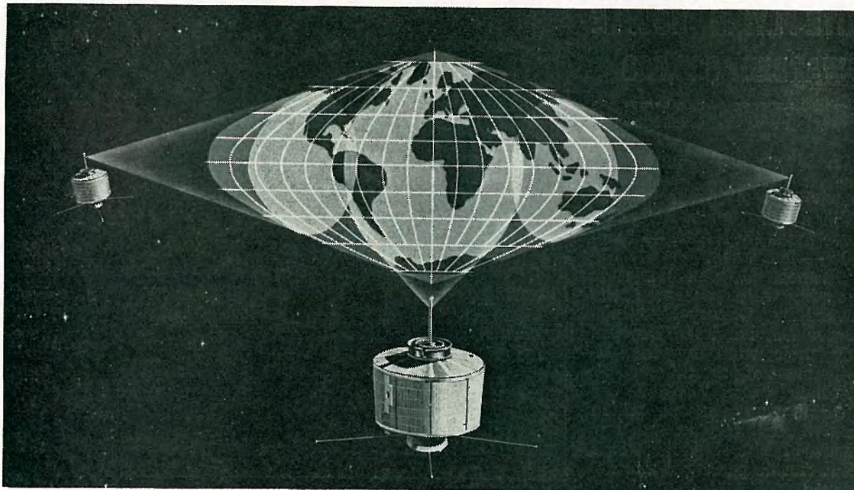
**DRAWING ILLUSTRATES** how three stationary type satellites can provide a global communications network with uninterrupted, 24-hour a day television and telephone service. Each Syncom satellite, at 22,300 miles altitude, can "see" a third of the globe. Microwave signals can be relayed via the satellites from any ground station to any other within the network. The satellites travel at a speed that is synchronized with the earth's rotation, and appear to hang motionless in the sky.
