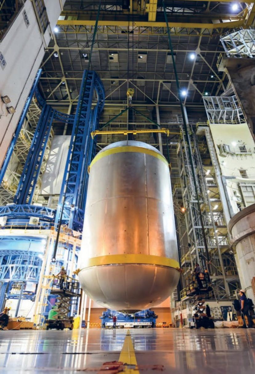
▲ This 196,000-gallon liquid oxygen tank, part of the system that will propel the Space Launch System rocket to lunar orbit, keeps the fluid at minus 297 degrees Fahrenheit.
