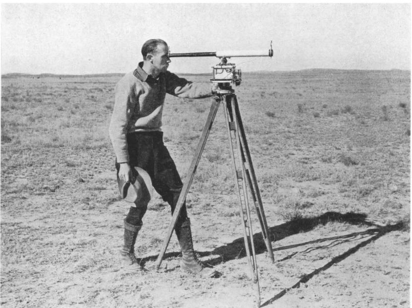
2. Observer stationed 3,000 feet from the tower with a recording telescope.
