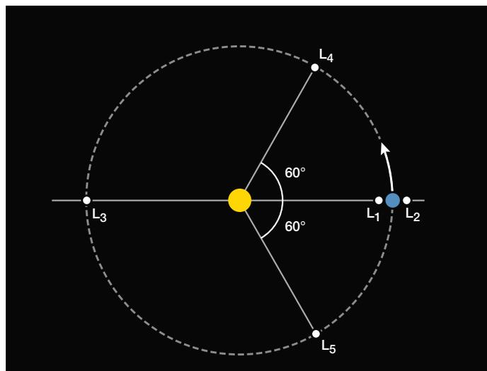
▲ **LAGRANGIAN POINTS** In a system of two massive bodies orbiting each other (such as the Sun and Earth), five gravitational “balance points” exist where a third, much smaller object can orbit in a constant pattern. A craft at  $L_2$  can always keep the Sun, Earth, and Moon behind itself, making it a frequent choice for space missions. Previous denizens of  $L_2$  include Europe's Planck and Herschel missions; the sky-scanning Gaia spacecraft is currently there.
