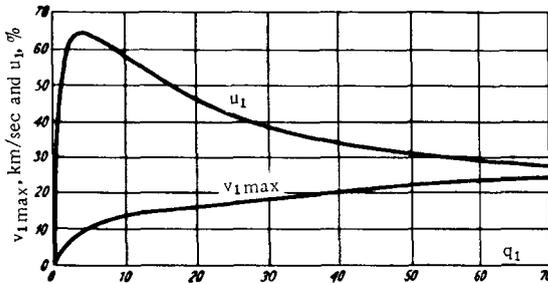
FIGURE 16. Flight velocity and utilization of the rocket.
