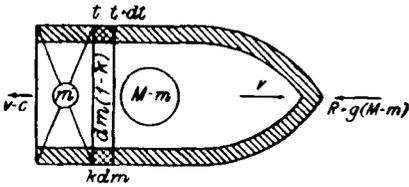
FIGURE 8. Deriving the equation of rocket motion
