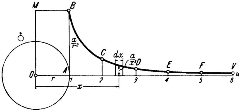
FIGURE 9. Variation in rocket weight with increase of its distance from the Earth
