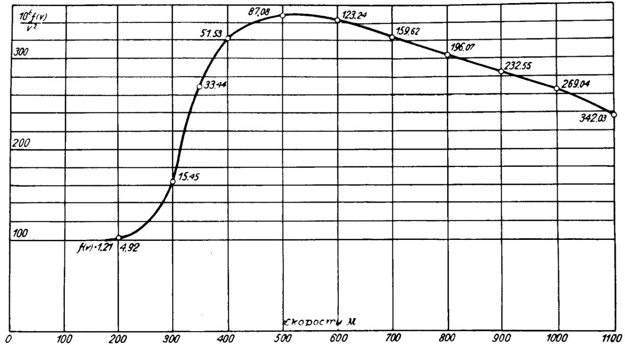
FIGURE 13. Curve of aerodynamic resistance
