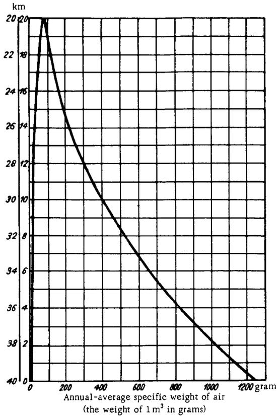
FIGURE 14. Change in weight of air with altitude
