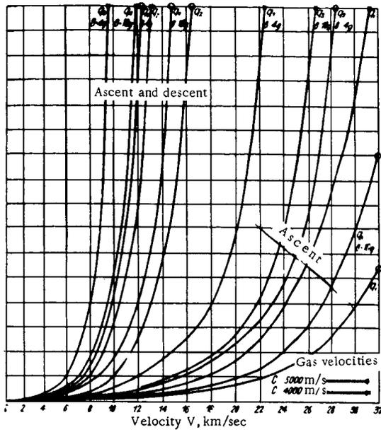
FIGURE 18. Rocket weights for different cases of rocket flight
