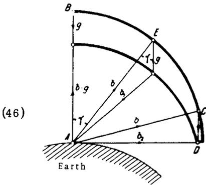
FIGURE 19. Inclined ascent of a rocket
