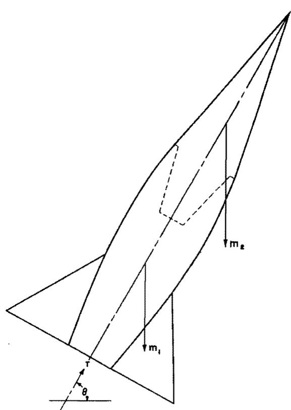
DIAGRAM - SATELLITE ROCKET LOADS AT SEPARATION
