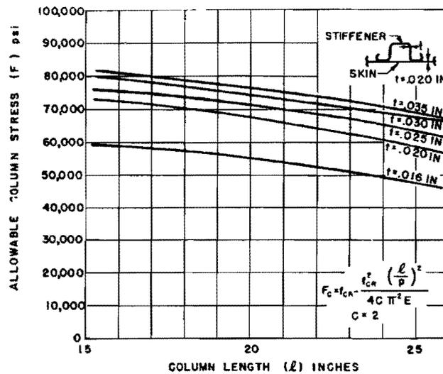
ALLOWABLE COLUMN STRESS vs COLUMN LENGTH FOR LONGITUDINAL STIFFENERS OF VARIOUS GAGES
