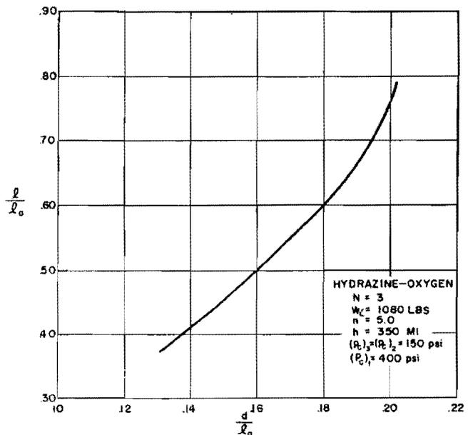
RELATION BETWEEN  $l/l_0$  AND  $d/l_0$  TO GIVE A SATELLITE ROCKET OF MINIMUM GROSS WEIGHT
