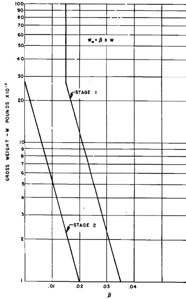
MISCELLANEOUS STRUCTURE WEIGHT FACTOR,  $\beta$ , vs GROSS WEIGHT
