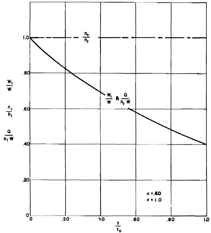
LOAD FACTOR, GROSS WEIGHT, AND APPLIED LOAD
