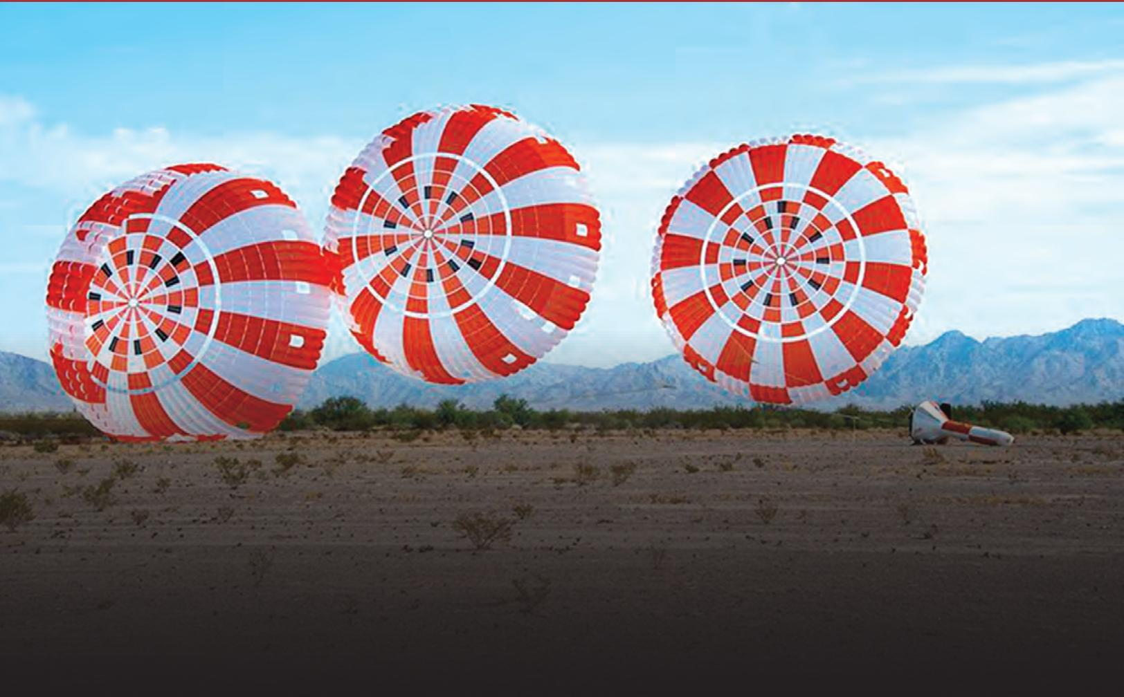
The parachute system for Orion, America's spacecraft that will carry humans to deep space, deployed as planned after being dropped from an altitude of 6.6 miles on July 12 at the U.S. Army Proving Ground in Yuma, Arizona. Data from the successful seventh drop in a series of eight qualification tests will help NASA engineers certify Orion's parachutes for missions with astronauts.
