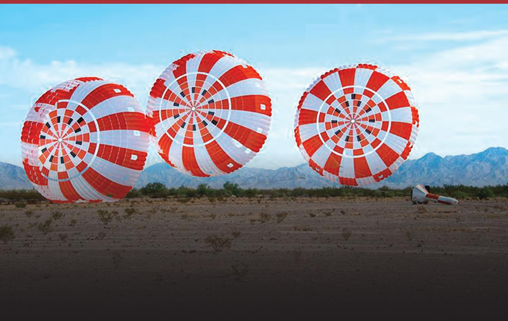
The parachute system for Orion, America's spacecraft that will carry humans to deep space, deployed as planned after being dropped from an altitude of 6.6 miles on July 12 at the U.S. Army Proving Ground in Yuma, Arizona. Data from the successful seventh drop in a series of eight qualification tests will help NASA engineers certify Orion's parachutes for missions with astronauts.
