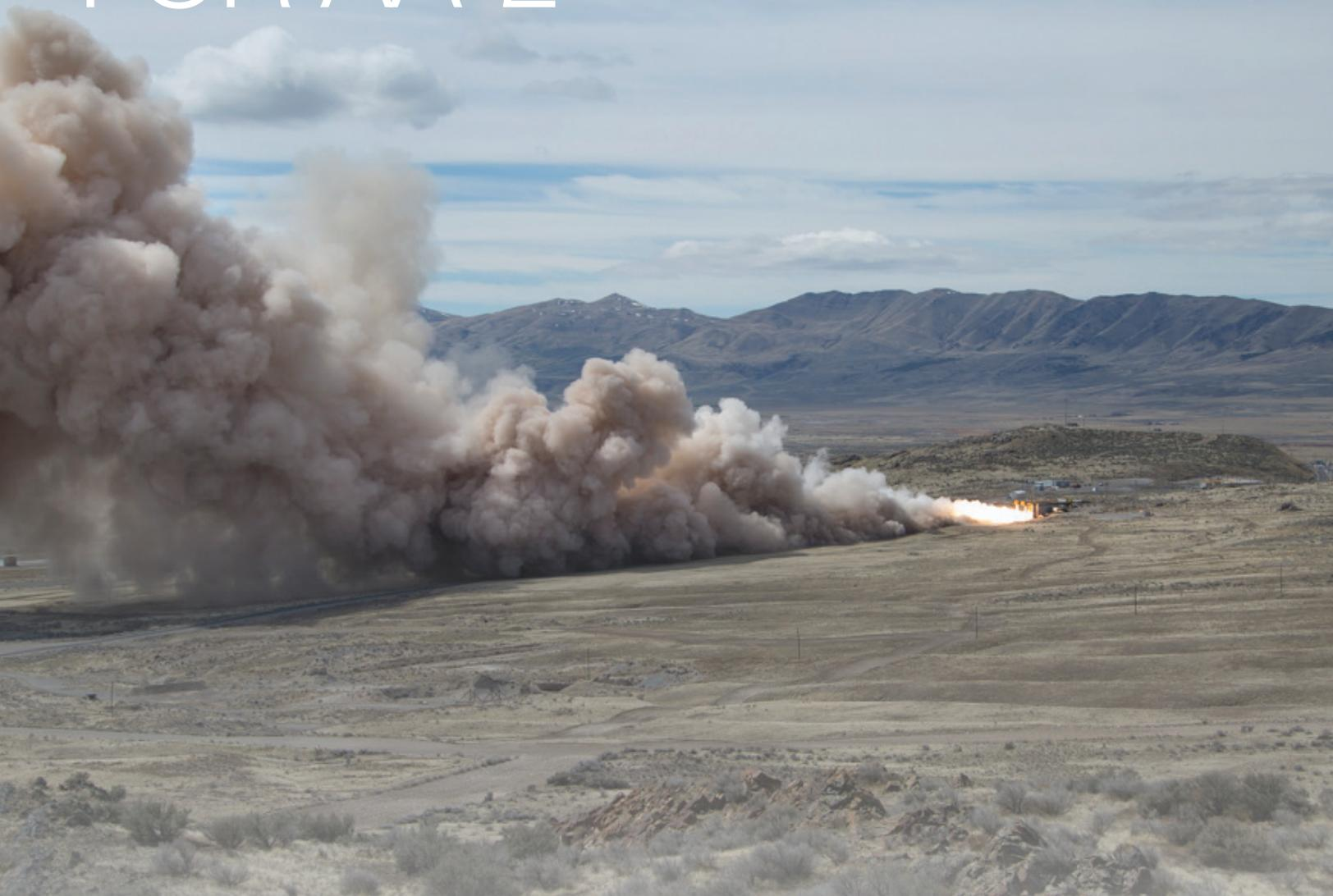
Orbital ATK successfully tested an SR 118 rocket motor at the company's Promontory, Utah, facility on March 29. Witnessing a rocket test or launch is exciting, and this one was no exception, as this ground test produced just the right amount of smoke and fire. NASA and Lockheed Martin will use an SR 118 rocket motor to launch an Orion test article to evaluate its Launch Abort System (LAS) in a test known as Ascent Abort-2, prior to launching a crewed Orion aboard NASA's Space Launch System.
