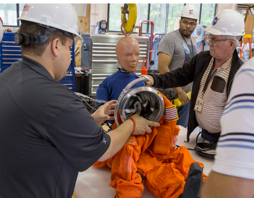
Engineers at NASA's Langley Research Center in Hampton, Virginia, dress a 105-pound representative female crash-test dummy into a modified Advanced Crew Escape Suit to prepare for water-impact testing at Langley's 20-foot-deep Hydro Impact Basin.
