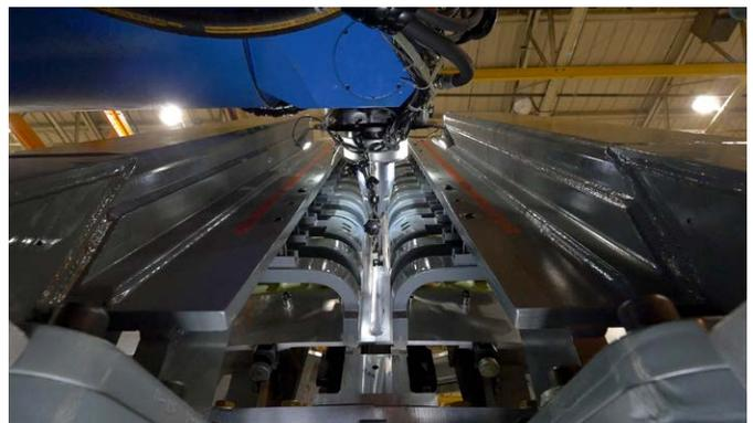
At NASA's Michoud Assembly Facility in New Orleans, engineers used large tooling structures to help them weld together Orion's cone panels using friction-stir welding.
