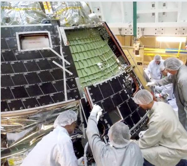
The Orion team at Kennedy Space Center's Operations & Checkout Building successfully completed the fit check on the back shell panels for the Orion vehicle prior to final installations in August.
