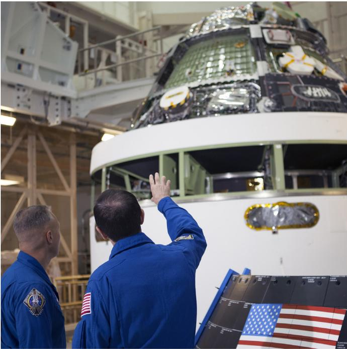
Astronauts Doug Hurley and Rex Walheim examine Orion and a section of the black back shell tiles that will be installed on the spacecraft now that the testing of the stacked crew and service module is complete.
