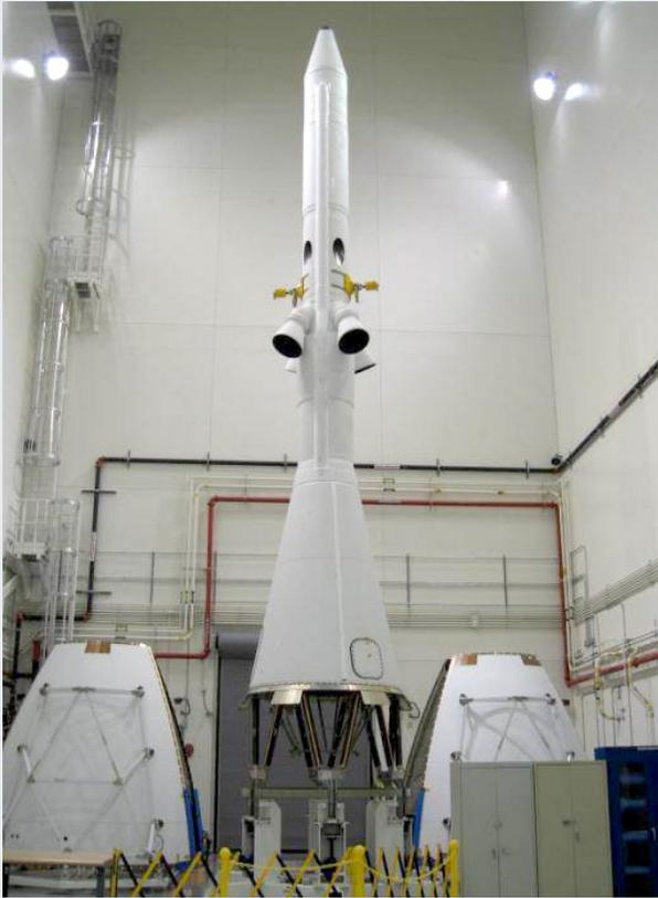
On July 25, the launch abort system was successfully uprighted from a horizontal to a vertical position on the assembly integration trailer and then transferred to the vertical support pallet in the Launch Abort System Facility at Kennedy Space Center in Florida.
