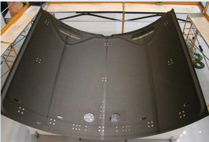
The Exploration Flight Test (EFT-1) Service Module fairing panels have been shipped to the Michoud Assembly Facility in New Orleans where they will be assembled as a tri-sector system.
