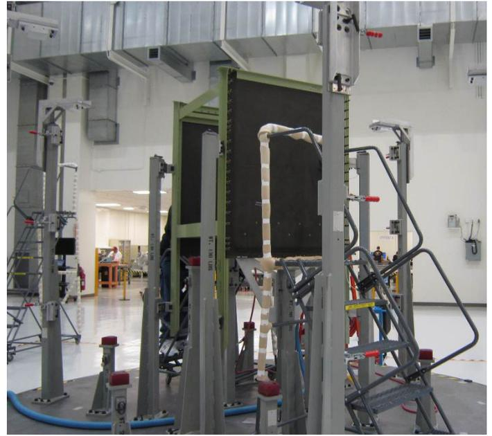
The team is also in the process of drilling and fastening the first two service module diamond panels to the shear web assembly structure.
