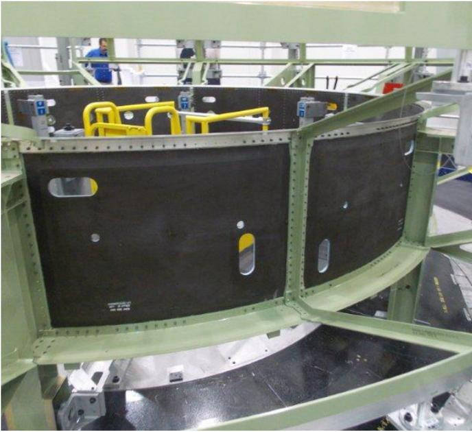
The team at Kennedy Space Center's Operations and Checkout building are in the process of wiring the thousands of sensors that will monitor the crew module's performance and are installing the aft gussets on the vehicle.
