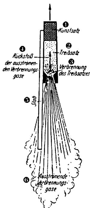
Figure 15. Fireworks rocket in a longitudinal section. The attached guide stick serves to inhibit tumbling of the rocket.
