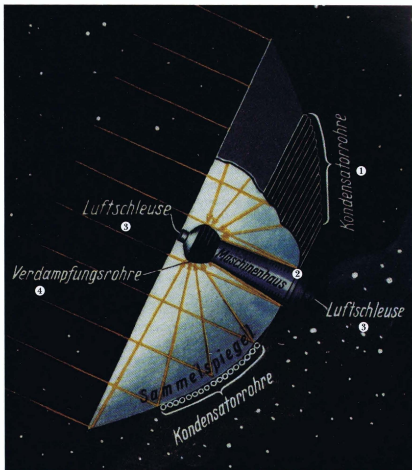
Figure 93. Example of the design of the machine room shown in the axial cross section.
