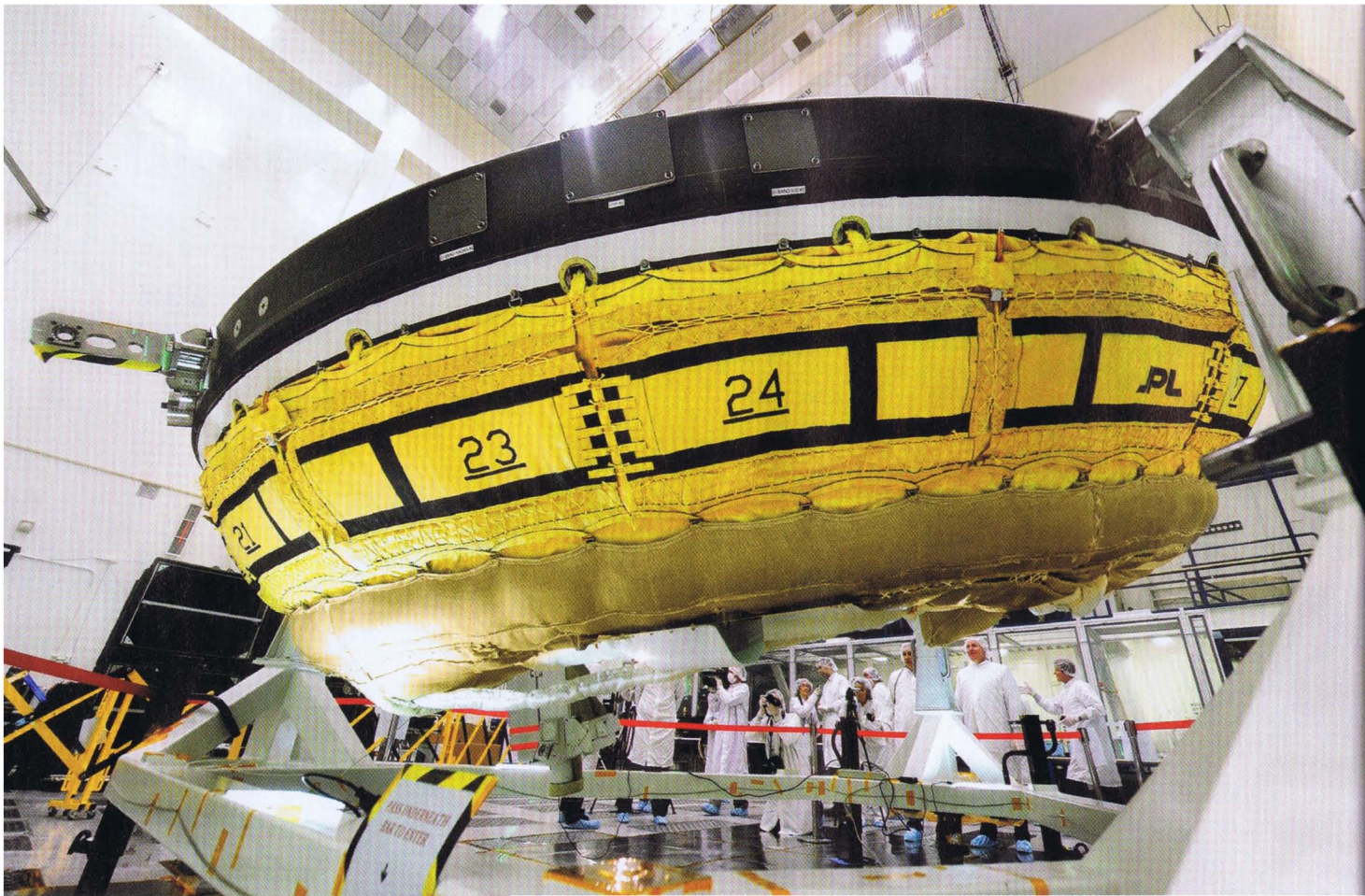
+ Journalists are briefed on NASA's Low Density Supersonic Decelerator in Pasadena, California. The project is aimed at enabling large payloads to be landed on the surface of Mars.
