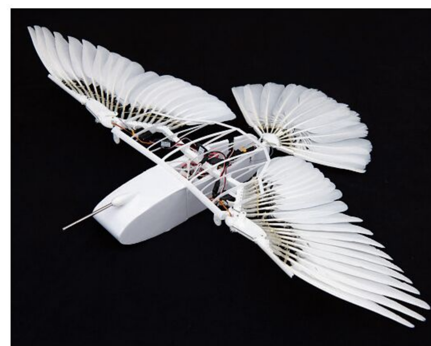
PigeonBot II, a robot designed to mimic the flying techniques of birds
