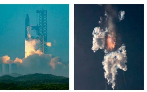
related to the failure of Starship and Super Heavy to disconnect from one another.
