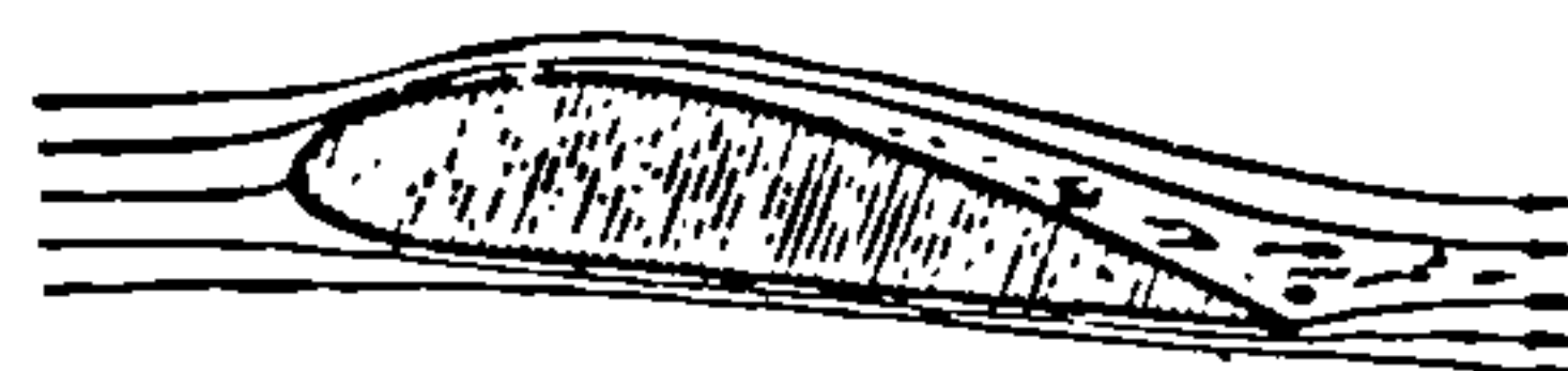
Fig. 14d. Subsonic flow around a wing profile; actual profile flow with region of dead space.
