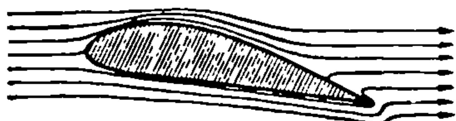
Fig. 14a. Subsonic flow around a wing profile; pure translation flow.
