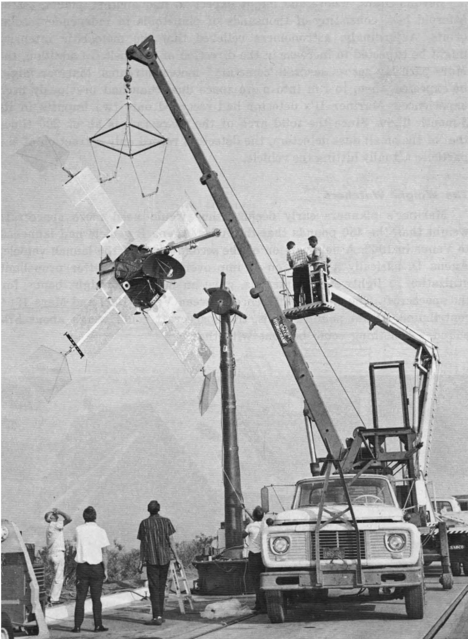
Preparations on antenna range for mapping actual characteristics of Mariner's two radio antennas
