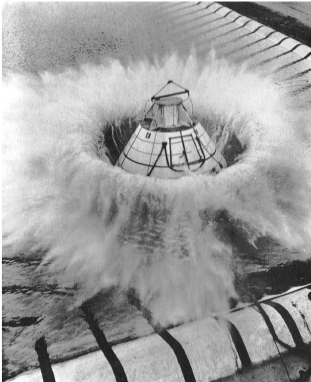
THE WATER IMPACT OF an Apollo boilerplate spacecraft at Downey provided a photographer with an opportunity for an unusual photo. The pendulum of the impact test facility there has been used extensively in tests and releases the spacecraft at controlled angles and speeds to simulate conditions the manned Apollo spacecraft will undergo on return to earth.
