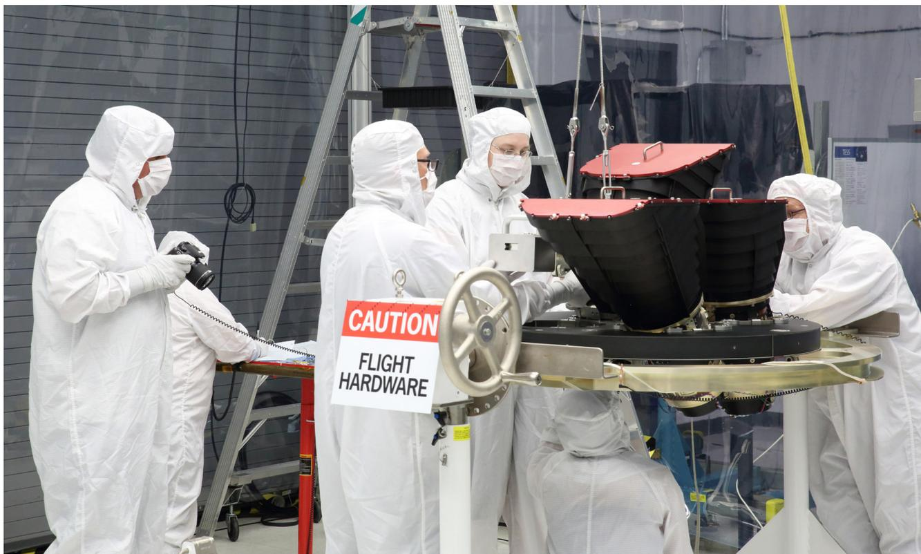
*Technicians mount the TESS cameras onto the camera plate in August 2017, prior to installation on the spacecraft. Orbital ATK*
