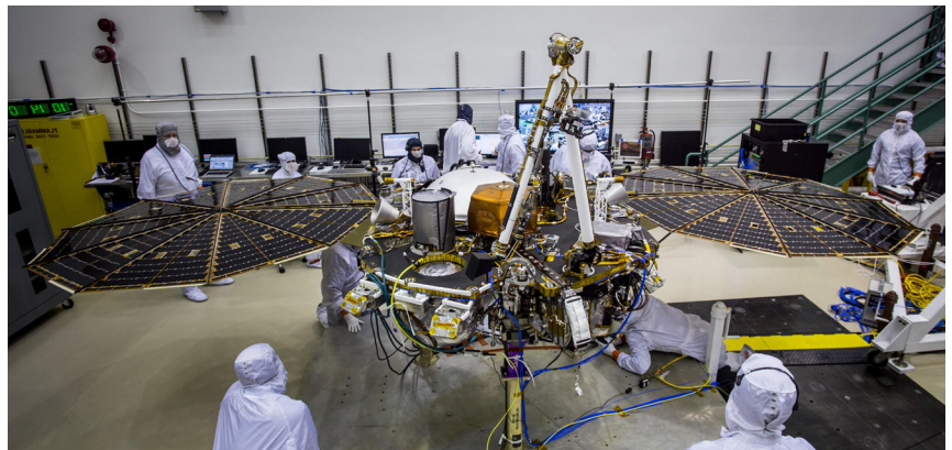
Engineers at Lockheed Martin Space, Denver, test the solar arrays on NASA's InSight lander several months before launch. Credit: NASA/JPL-Caltech/Lockheed Martin Space
