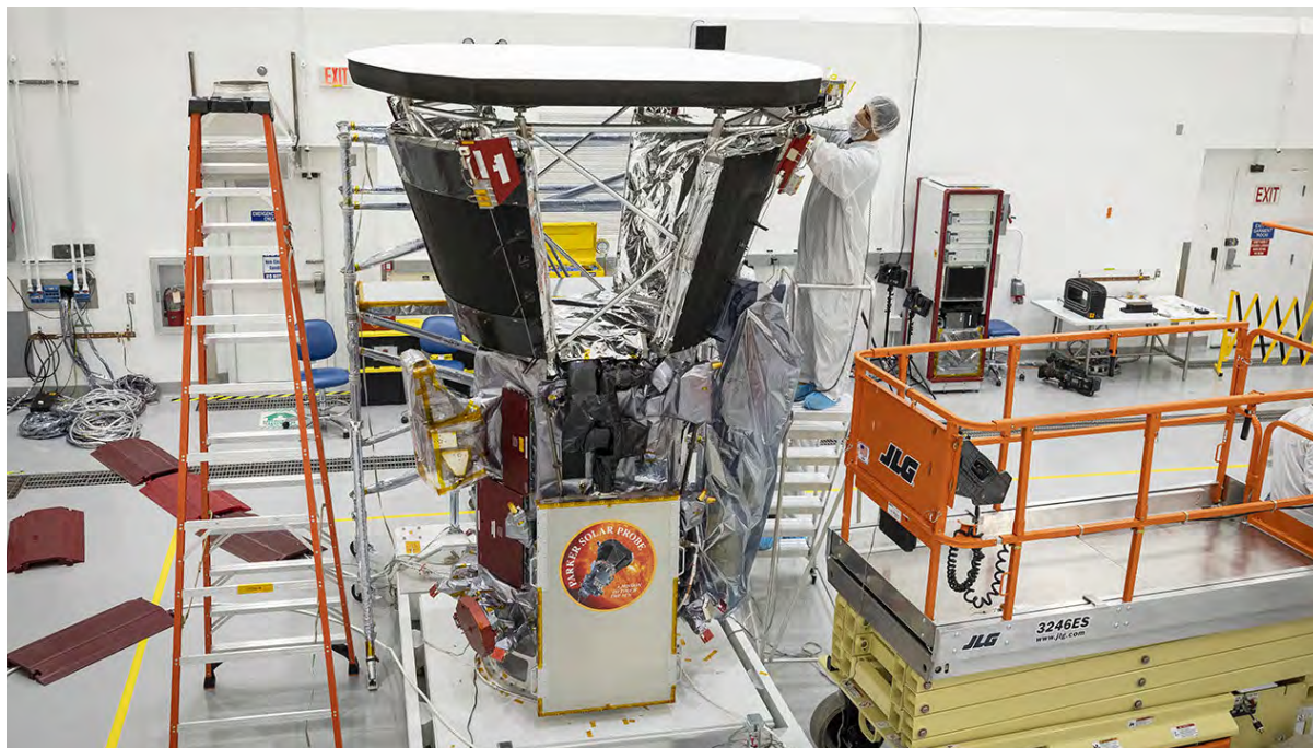
Parker Solar Probe's heat shield was installed on the spacecraft on June 27, 2018.
