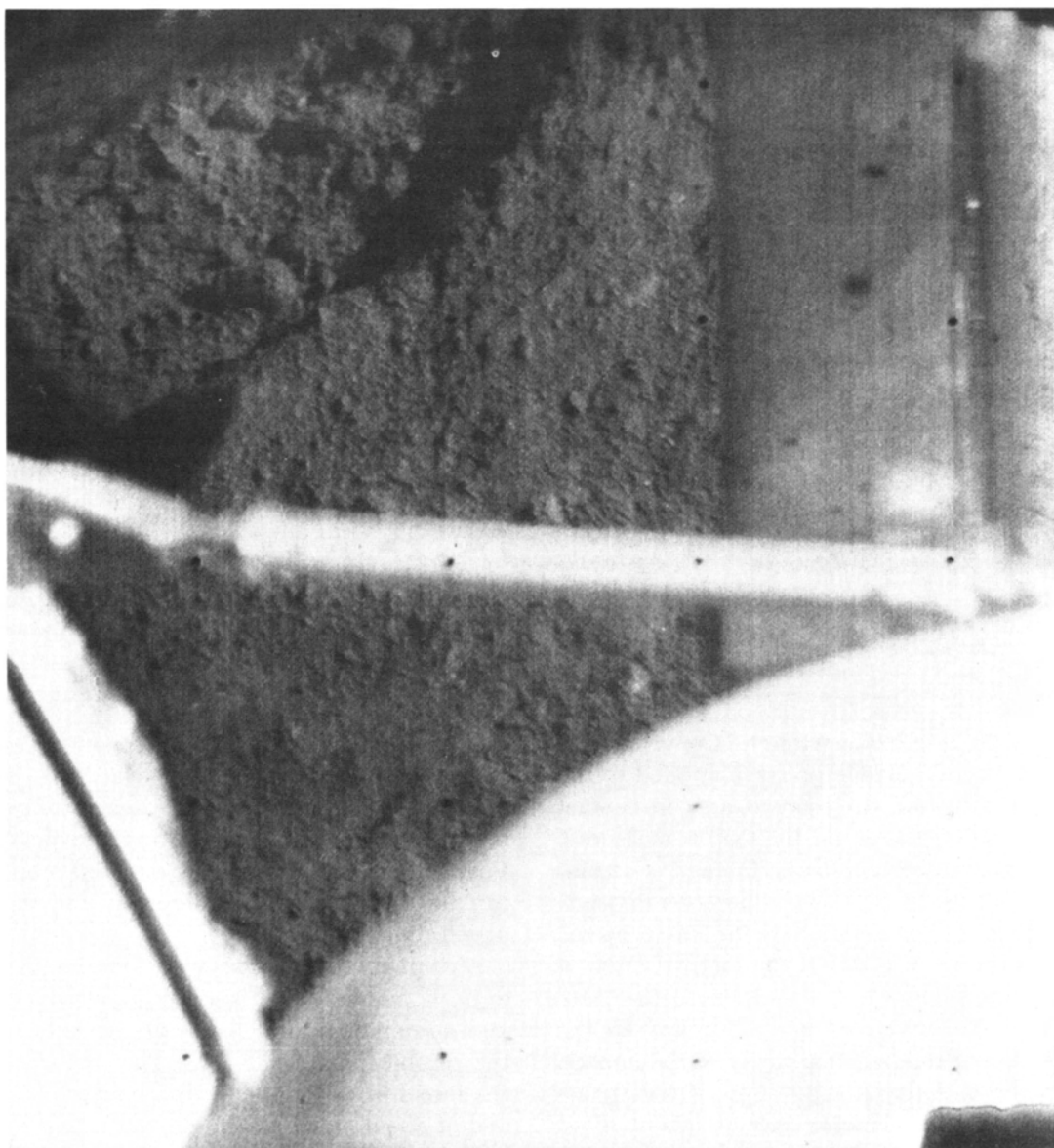
FIGURE 11.— Photograph of the surface depression made by crushable block 3. Note the depression made in the upper left-hand corner. Some parts of the spacecraft are shown.
