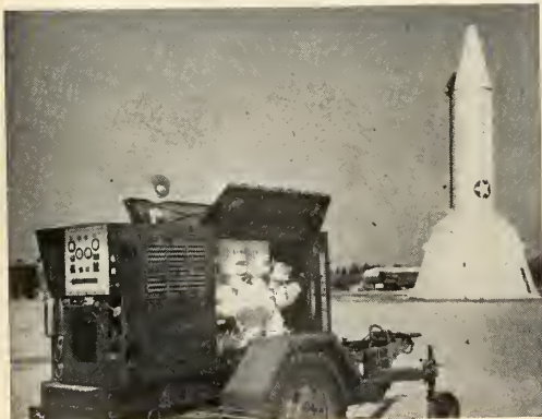
TWO IMPORTANT items for Jupiter: 100 KW power generator and vertical check-out shelter.
