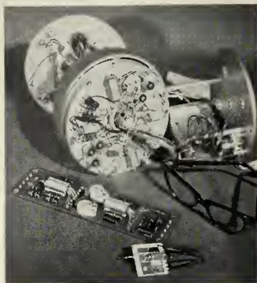
CONVENTIONAL wired subcarrier oscillator is shown at rear, printed circuit chassis in the middle, and a subminiature printed component device at front.
