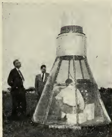
FULL-SCALE model of Project Mercury antenna fairing under test by Collins Radio engineers. Complete communication system, scheduled for delivery this month, is being built by Collins for McDonnell Aircraft. It consists of 14 electronic subsystems providing pilot voice communication during orbit; command functions within capsule for all phases; telemetry during all phases; tracking during orbit; voice communication and beacons for recovery/rescue; plus antennas.
