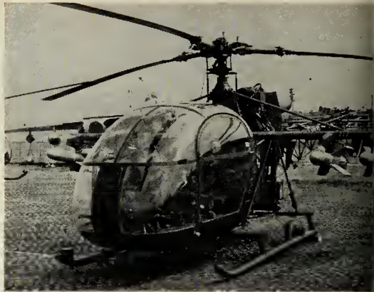
FRENCH Nord SS-11 air-to-ground anti-tank bird attack missile mounted on Sud Aviation helicopter. Photo by René Saint-Paul.
