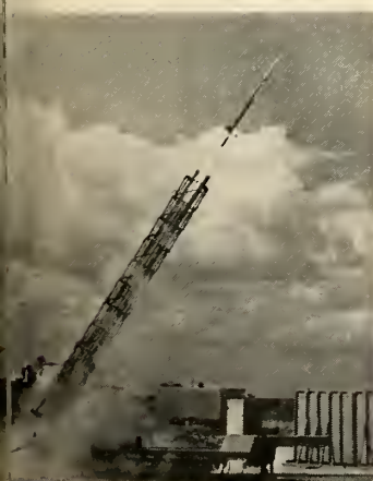
TAKE-OFF from Wallops Island, end-burning Arcon has high acceleration.
