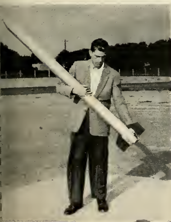
LIGHTNESS and ease of handling for ARCAS , 72-pound research rocket is design requirement.
