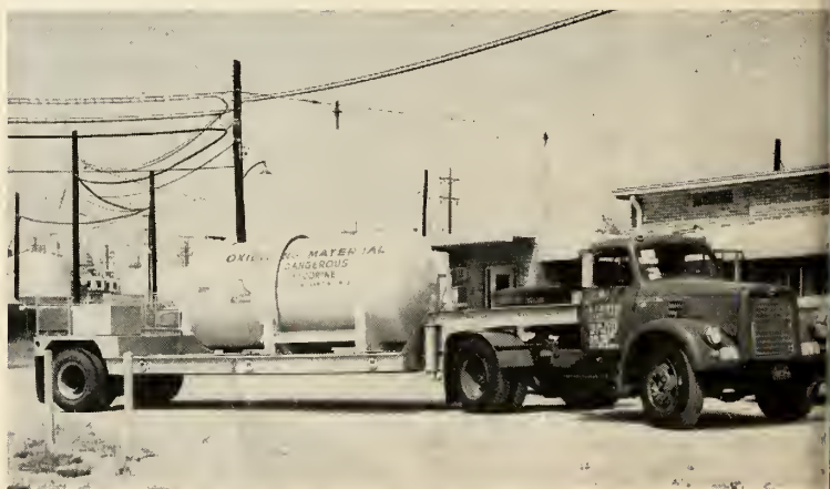
FEASIBILITY of transport of large quantities of highly-toxic liquid fluorine has been demonstrated by Allied Chemical.
