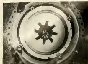
AP aluminized propellant made it possible to pour directly into 13-foot case without benefit of rubber liner.
