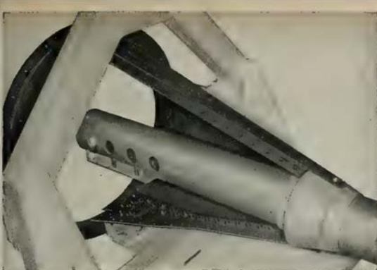
NOSE CONE SPLICE JOINTS ARE FASTENED WITH HS67 PINS, TYPE 431 STAINLESS STEEL, HEAT TREATED TO 125,000 PSI MINIMUM SHEAR. THE HS60M COLLARS ARE R MONEL.
