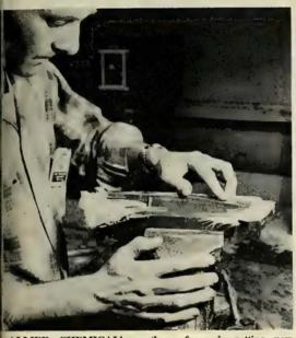
ALLIED CHEMICAL's urethane foam is getting new use as material for wind tunnel test models, particularly at Chance Vought. Open mold is lined with glass cloth and epoxy resin laminated before foam is poured. The smooth skin offers less drag, and is cheaper than wooden surface models.
