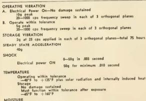
Operate within tolerance Relative humidity up to 95% may include condensation
